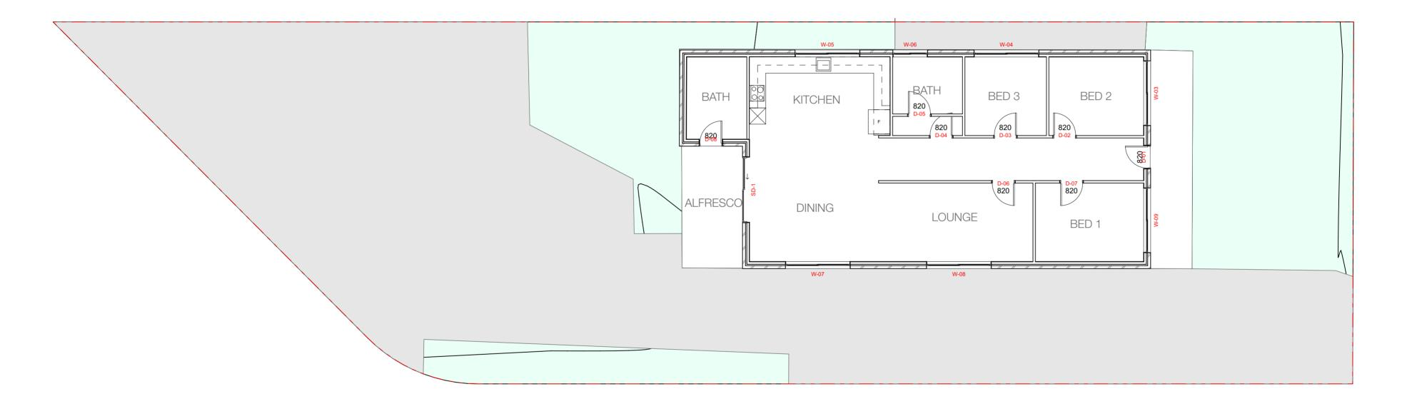
SMOKE ALARMS TO BE COMPLIED CLAUSE 9.5.4 OF THE NCC VOLUME TWO 2022 & AS3786:2014 - WATERPROOFING IN ALL WET AREAS TO BE INSTALLED IN ACCORDANCE WITH AS3740 OR AS3740 AND PART 10.2 OF THE ABCB HOUSING PROVISIONS - ALL MECHANICAL VENTILATION SYSTEMS TO BE COMPLIED WITH BCA PART H4D9 AS REQUIRED BY THE
